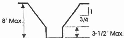
Figure 3. Type A Soil Unsupported, Vertically Sided Lower Portion, Maximum 8 Feet in Depth
